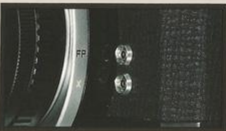
● Two CdS cells incorporated for activating the exposure meter, and an extra CdS for Photoswitch on top.
